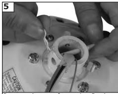
Remove keeper from pin. Replace keeper into pin and save for later.
